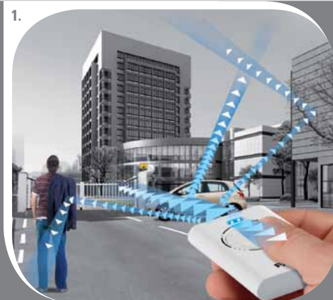
1. Standard transmitters: the surrounding environment, including the user's hand, changes the radio emission and only a part of the transmitted power reaches the receiver.
